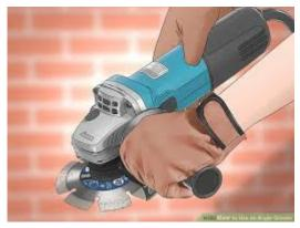
large for the tool. The stone's maximum RPM. rating was also lower than the grinder's. As the worker started to grind, the stone broke, and pieces of stone struck and injured him.
