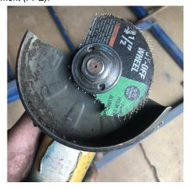
Angle grinders have several functions including sanding, grinding and cutting processes, depending on the type of disc used. When operating, the cutting or grinding disc may come into contact with a body part, or shatter and throw off pieces at extremely high speed. An operator could easily sustain cuts, abrasions, burns or eye injuries.
