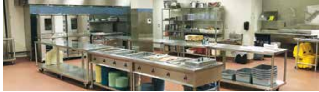
Finished kitchen, designed to accommodate groups of 20 people. It features a slip-resistant, impact-resistant, waterproof floor, and everything is stainless steel and on wheels.
