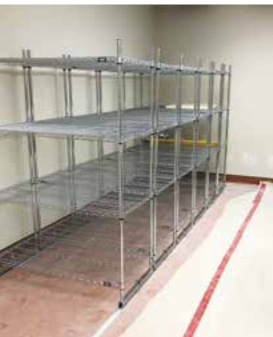
Sliding shelves. The shelves sit on runners and are held down by their own weight, so they don't puncture the floor.
