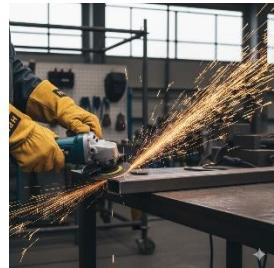
Another worker was cutting part of a structure with a grinder and a zip cut wheel. The wheel bound and broke; a piece flew off, striking the worker's arm. The zip cut wheel was the correct type and size for the tool, and the worker was wearing the appropriate personal protective equipment (PPE).
